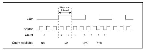
Figure 2-16. Single Pulse Width Measurement
